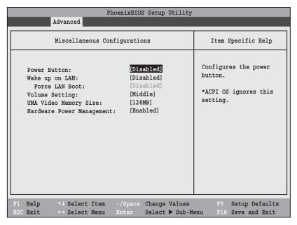
Figure 10. Miscellaneous Configurations Submenu
